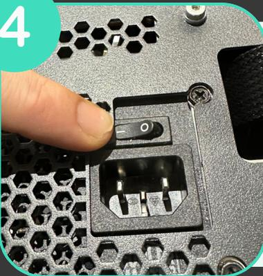
Make sure the power supply is in the "ON" position
