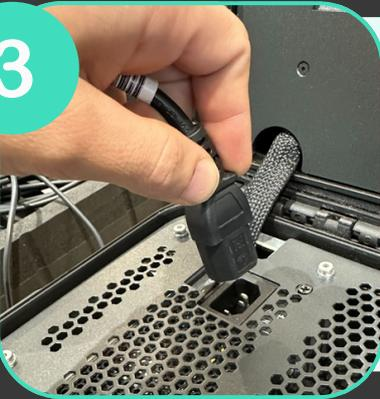
Connect the power supply to an electrical socket
