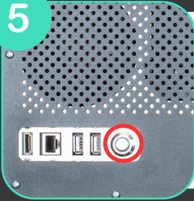
Press the power button on the front of the case (the button lights up when the computer starts)
