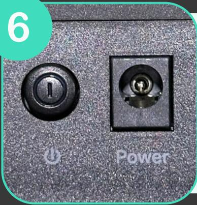
Make sure that the router (included as an option) is plugged in and that the "ON" position is engaged.
