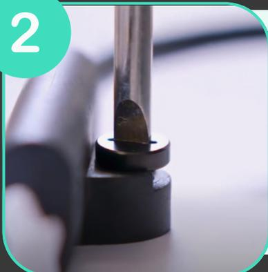
Screw the USB-C port onto the device using the small screwdriver supplied in the box
