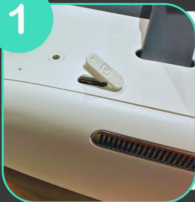
Lift the small cover with the letter "D" and connect the USB-C cable to your headset
