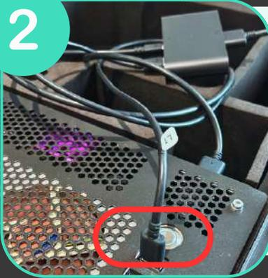
Connect your Linkbox (Usb and DisplayPort) to your computer and to an electrical socket (electricity)
