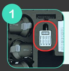
Insert your batteries into the built-in charger in the case
