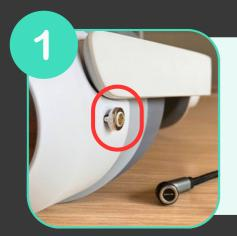
Make sure the magnetic tip is properly connected to the headset.
