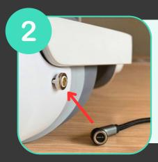
Hold the magnetic cable close to the end cap to recharge your headset.
