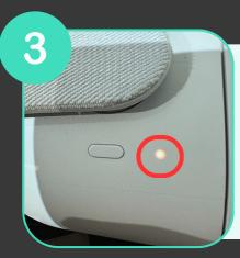
Make sure the headset is charging by checking the LED on the headset\*.
